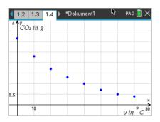
Solubility of carbon dioxide in g per liter of water as a function of temperature at p = 1 bar
