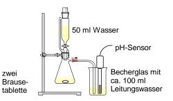
Prepare data acquisition so that a reading is taken every 5 seconds over a period of 300 seconds.
