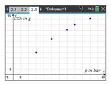
Solubility of carbon dioxide in g per 1 liter of water as a function of pressure at a temperature of  $\vartheta$  = 20 °C.
