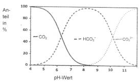
pH dependence of carbon dioxide, hydrogen carbonate and carbonate equilibrium in aqueous solution Werte nach: https://link.springer.com/chapter/10.1007/978-3-642-17813-9\_3
