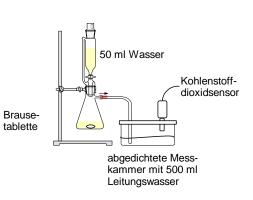
Prepare the computer with connected  $CO_2$  sensor for data acquisition in such a way that a measurement value is recorded every 10 seconds for a period of 600 seconds. Start the data acquisition. After approx. 30 seconds, open the tap on the dropping funnel so that water is directed drop by drop to the effervescent tablet and carbon dioxide is slowly introduced into the water.
