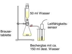
Prepare the computer with connected conductivity sensor (measuring range 200  $\mu$ S) for data recording so that a measured value is recorded every 5 seconds for a period of 300 seconds.
